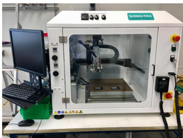
Figure 4.3. Photographic image of the ultrasonic spray-coating device (Exactacoat, Sono-Tek) used for electrode fabrication.
